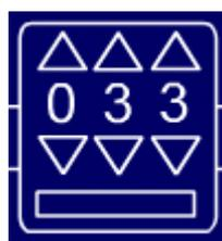
Inlet and outlet controls can be set using the pointers. This is set to let 33 units of liquid flow out of the measuring cylinder once the tap is turned.
